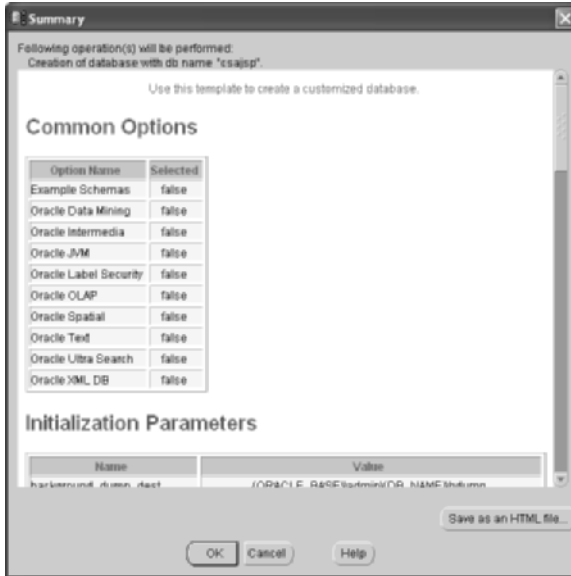
Figure 18–28 Tenth DBCA window: summarizes the configuration options before the database is created.
