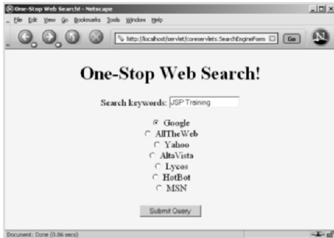
Figure 6–3 Front end to the SearchEngines servlet. See Listing 6.5 for the source code.
