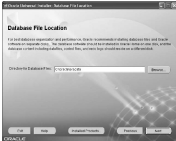
Figure 18–12 Ninth Oracle install window: for specifying the physical location of the database.
