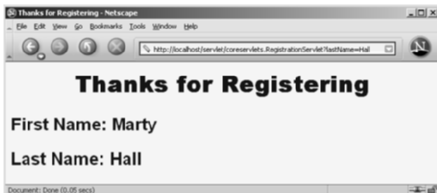
Figure 15–8 Result of RegistrationServlet when one parameter is missing and session data is found.
