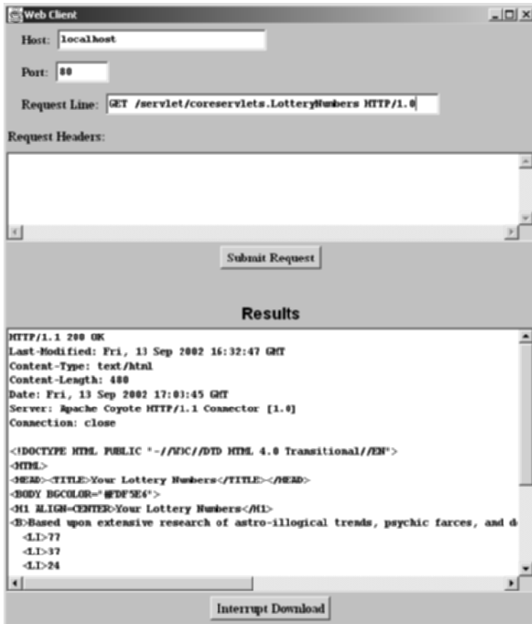
Figure 3-7 Accessing the LotteryNumbers servlet results in normal response (with the document sent to the client) in two situations: when there is an unconditional GET request or when there is a conditional request that specifies a date before servlet initialization. Code for the WebClient program (used here to interactively connect to the server) is available at the book's source code archive at http://www.coreservlets.com/ .
