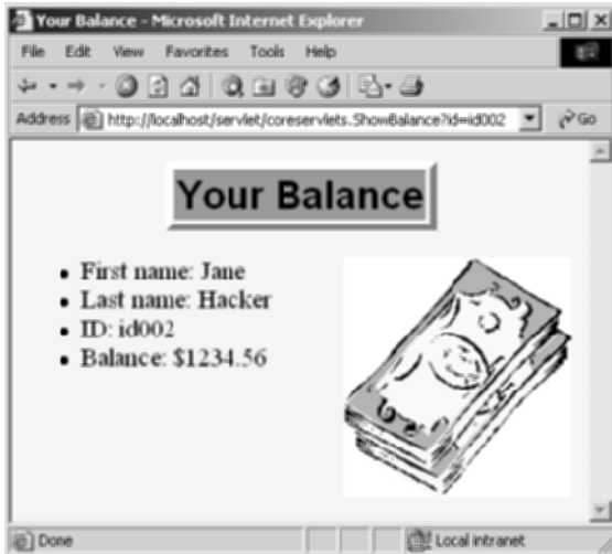
Figure 15–3 The ShowCustomer servlet with an ID corresponding to a customer with a normal balance.
