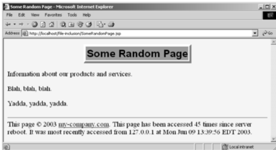
Figure 13–2 Result of SomeRandomPage.jsp . It uses the include directive so that it maintains access counts and most-recent-hosts entries separately from any other pages that use ContactSection.jsp .
