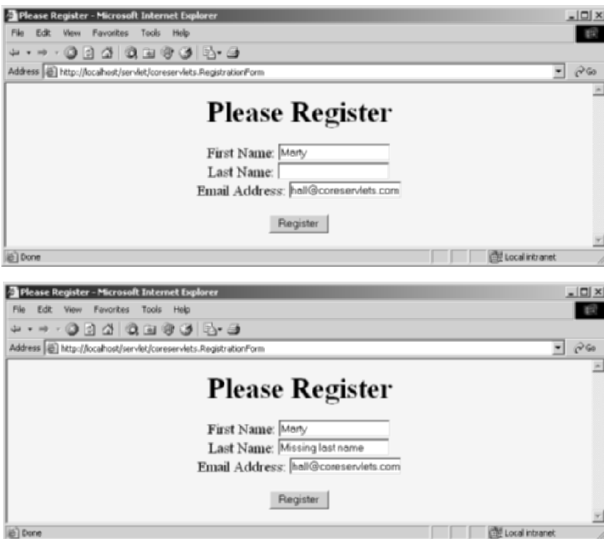
Figure 8–12 When the input form is incompletely filled in (top), the RegistrationServlet redirects the user to the RegistrationForm (bottom). The RegistrationForm uses cookies to determine the values of the form fields that were already filled in.
