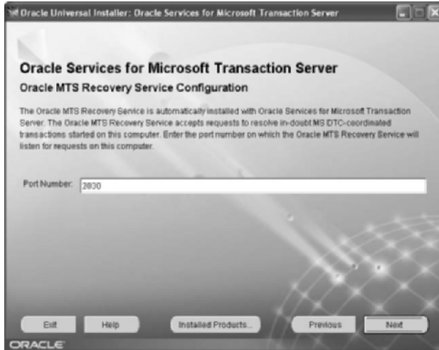
Figure 18–10 Seventh Oracle install window: for specifying a port for the Oracle MTS Recovery Service.
