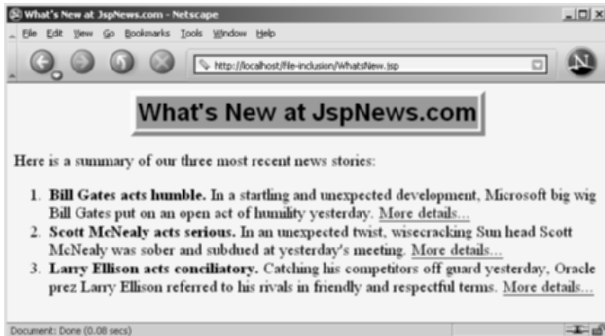
Figure 13–1 Including files at request time lets you update the individual files without changing the main page.
