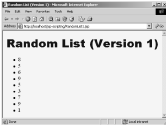
Figure 11-12 Result of RandomList1.jsp . Different values (and a different number of list items) are displayed whenever the page is reloaded.
