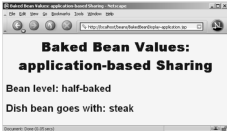
Figure 14–15 Subsequent request to BakedBeanDisplay-application — BakedBean properties persist between requests even if the request is from a different client (as here) or is in a different session.
