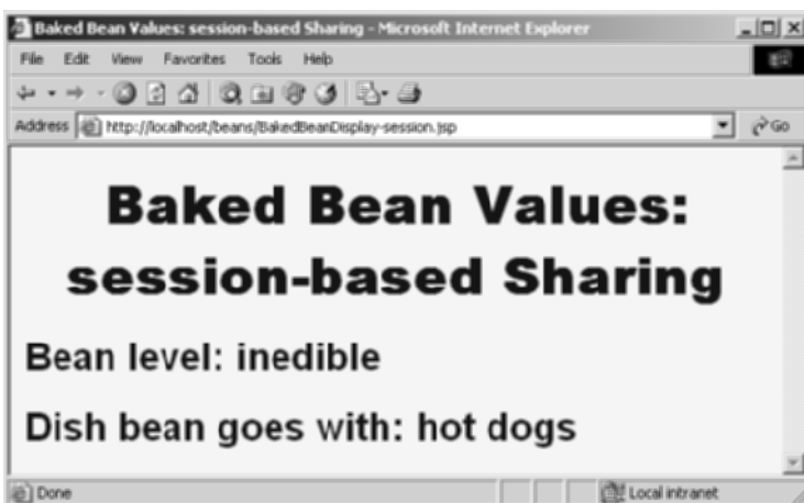
Figure 14–11 Subsequent request to BakedBeanDisplay-session.jsp—BakedBean properties persist between requests if the request is from the same client in the same session.
