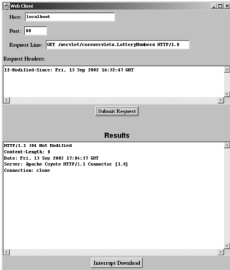
Figure 3–8 Accessing the LotteryNumbers servlet results in a 304 (Not Modified) response with no actual document in one situation: when a conditional GET request is received that specifies a date at or after servlet initialization.
