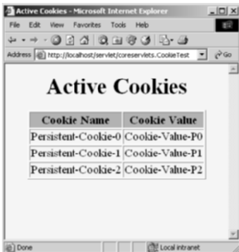
Figure 8-7 Result of revisiting the CookieTest servlet within an hour of the original visit, in a different browser session (browser was restarted between the original visit and the visit shown here).
