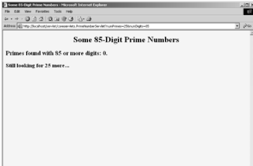
Figure 7-3 Initial results of the prime-number-generation servlet. A quick result is sent to the browser, along with instructions (in the Refresh header) to reconnect for an update in five seconds.
