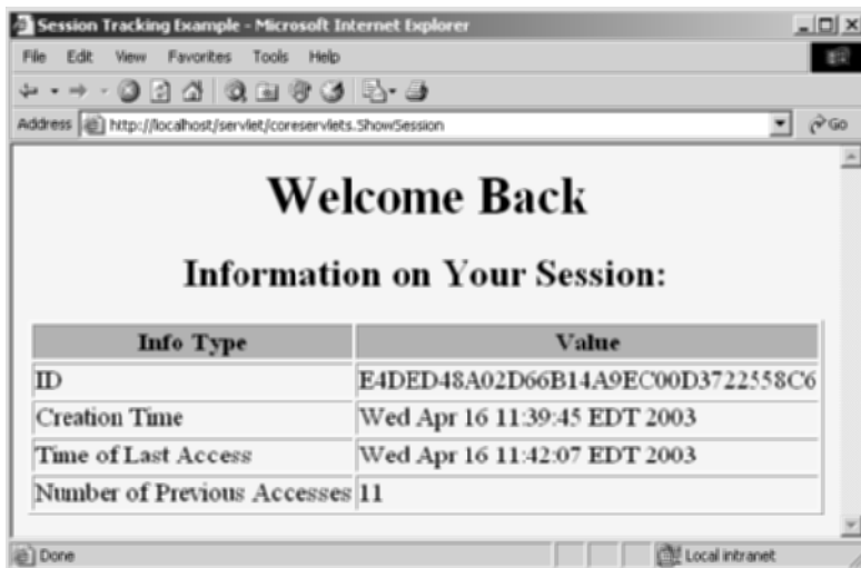
Figure 9-2 Twelfth visit to ShowSession servlet. Access count for this client is independent of number of visits by other clients.
