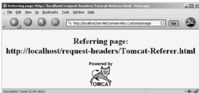
Figure 5–8 The CustomizeImage servlet when the address of the referring page contains neither “JRun” nor “Resin.”
