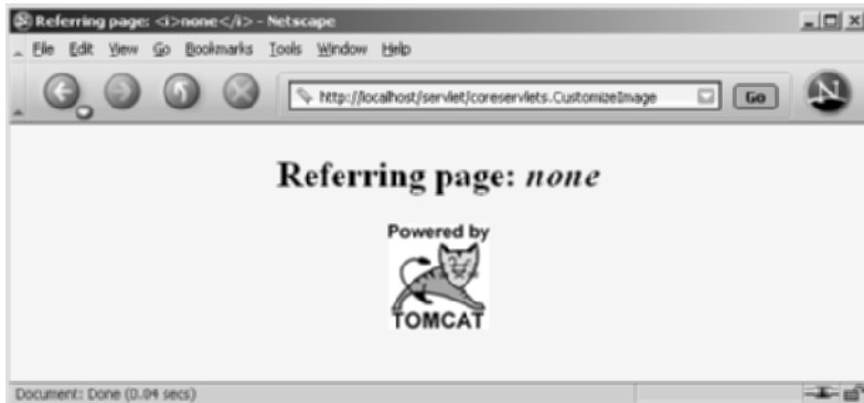
Figure 5-9 The CustomizeImage servlet when the Referer header is missing. When using the Referer header, always handle the case in which the result of getHeader is null .
