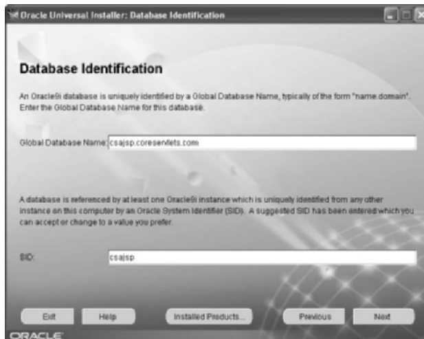
Figure 18–11 Eighth Oracle install window: for specifying the name of the global database and SID.
