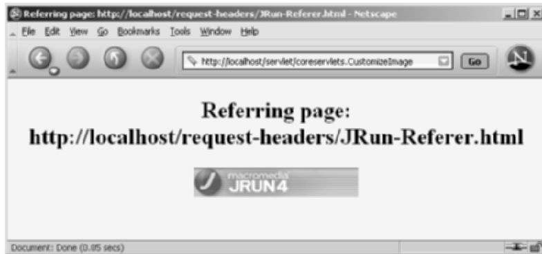
Figure 5–6 The CustomizeImage servlet when the address of the referring page contains the string “JRun.”
