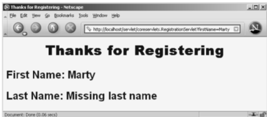
Figure 15-7 Result of RegistrationServlet when one parameter is missing and no session data is found.
