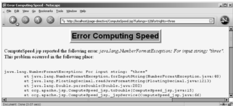
Figure 12–8 ComputeSpeed.jsp when it receives illegal values. Note that the address line shows the URL of ComputeSpeed.jsp, not SpeedErrors.jsp.
