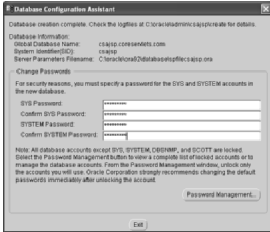
Figure 18–17 Fourteenth Oracle install window: for specifying passwords. Use the Database Configuration Assistant to specify a password for the SYS and SYSTEM administrative accounts.
