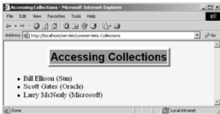
Figure 16–4 You use array notation or dots to access collections. Dots can be used only when the key is in a form that would be legal as a Java variable name.
